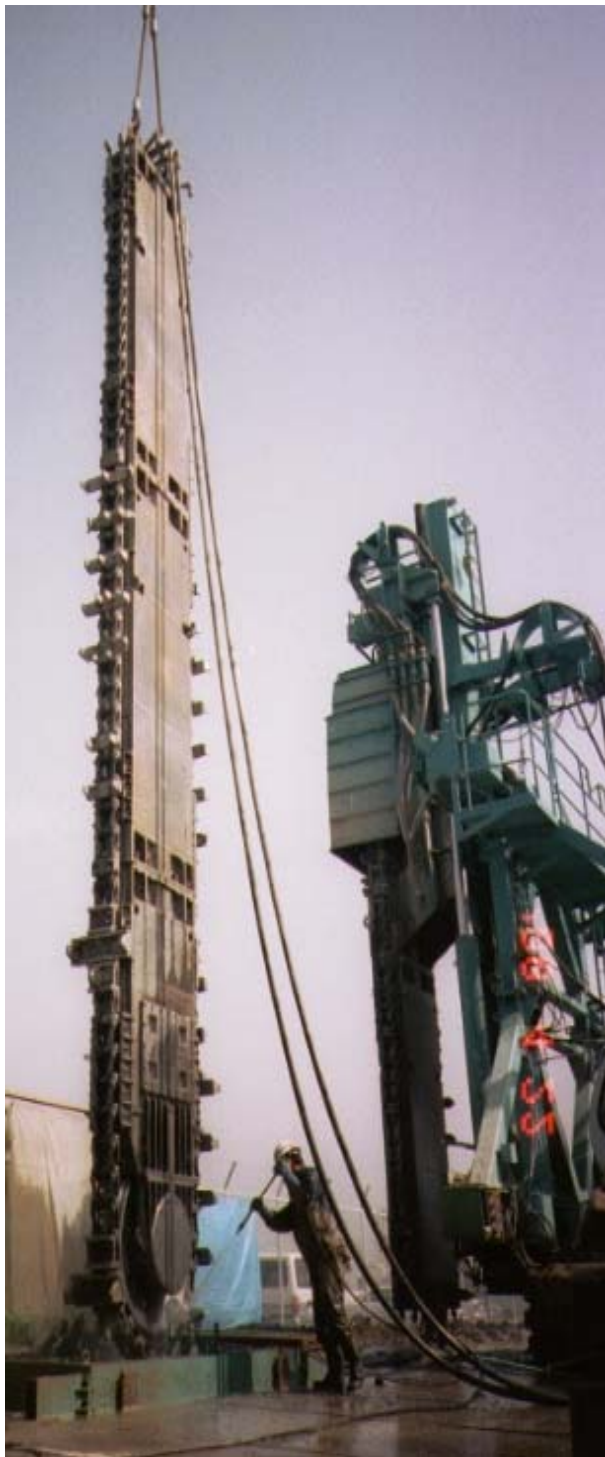
Figure 3. TRD “Cutting Post,” showing the cutting chain. (TRD promotional information.)
