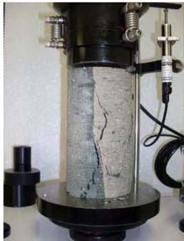
Figure 8 . Compression test on a cored inter-element sample.
