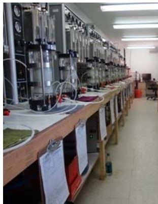
Figure 9. Hydraulic conductivity testing of wet grab samples (Category 1 wall).
